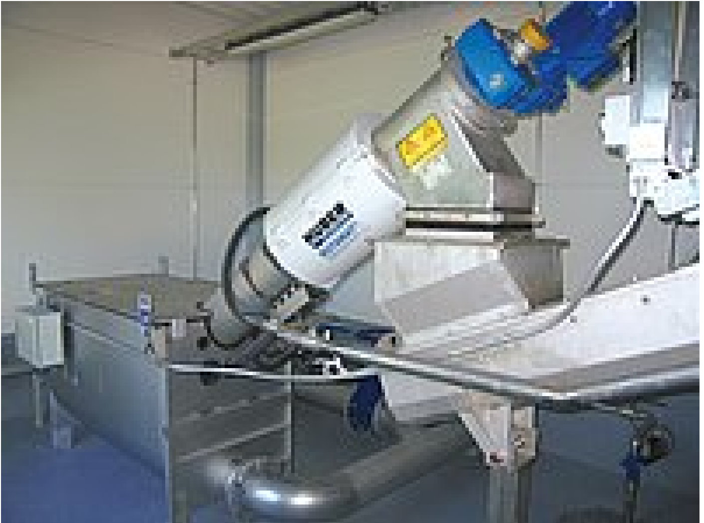
Septage receiving station Ro 3 with integrated IRGA for screenings washing and enclosed Ro 8t screw conveyor forwarding the screenings to wash-press WAP/SL
