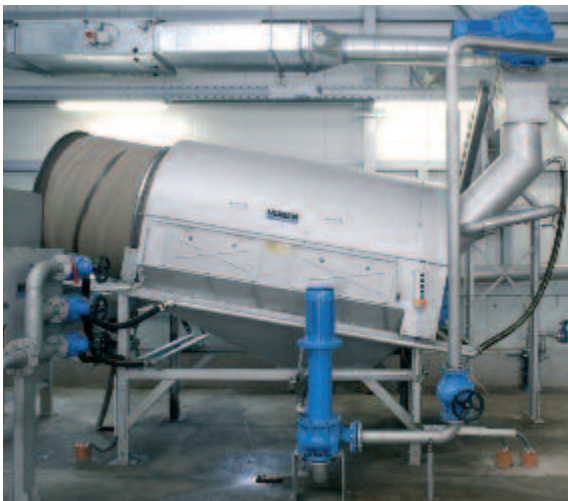
ROTAMAT® Wash Drum for washout and separation of all coarse material > 10 mm
