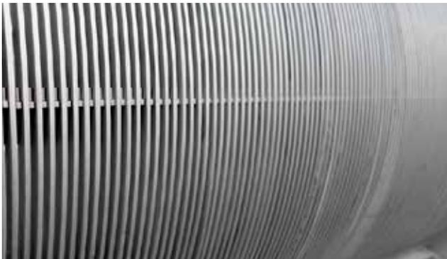
*The rake tines, fully engaging with the bar rack, prevent jamming of solids in the bar spacings.*
