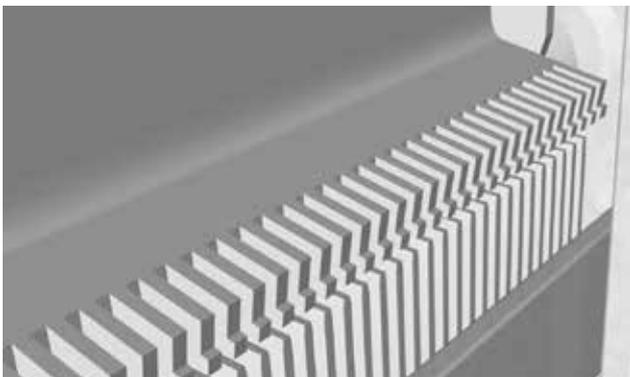
*Moreover, the screen proves its insensitivity to abrasive materials, such as grit and gravel, as the screen rake engages above the bar rack.*
