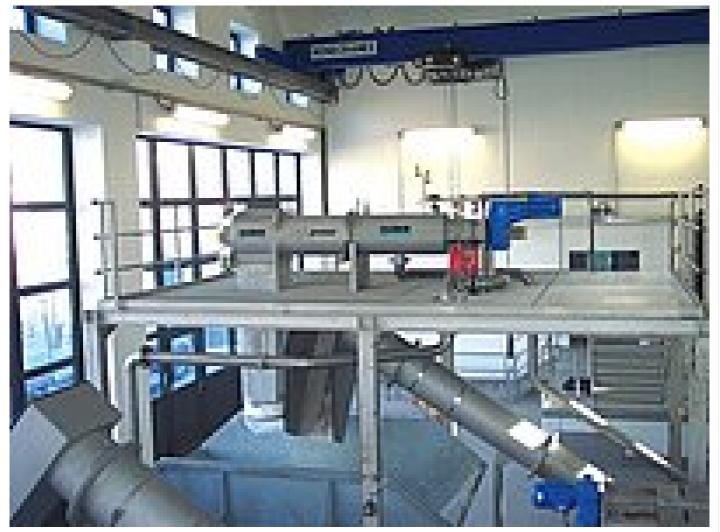
Coarse material separator for municipal and industrial sludge and process water
